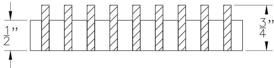
Drop in core which can be used for multiple applications where either blocking, wood work, angle or support is in place for the core to rest upon.
