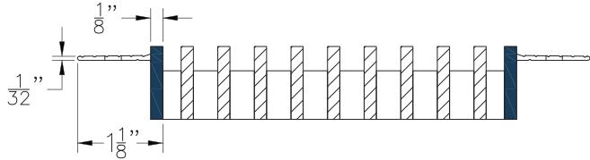
J-Bead Frame for wall and ceiling applications with fixed core.
