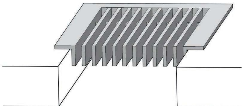
Drop in B Frame typically used for a rough cut opening since the flange provides a crisp, clean, finished appearance.
