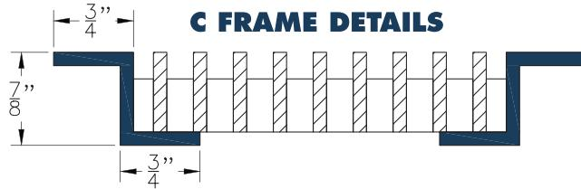
C Frame drop in typically used for floor and sill applications.
