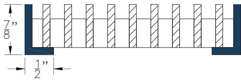
Drop in A Frame typically used for an enclosure, fin tube opening, floor vents and millwork.
