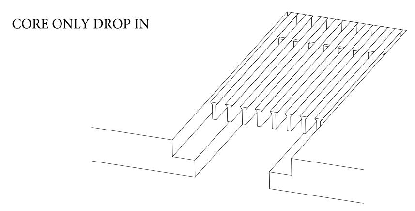
Drop in core which can be used for multiple applications where either blocking, wood work, angle or support is in place for the core to rest upon. Used on sills, radiators and enclosure covers.
