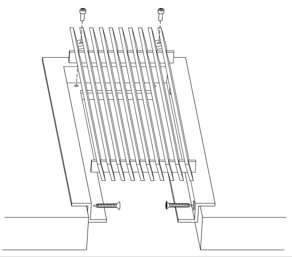
Always with removable core – C Frame with concealed, countersunk mounting holes on the inside of frame for fastening to the opening.
