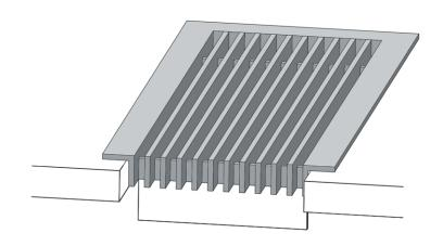
14. B FRAME Inverted with mounting holes
